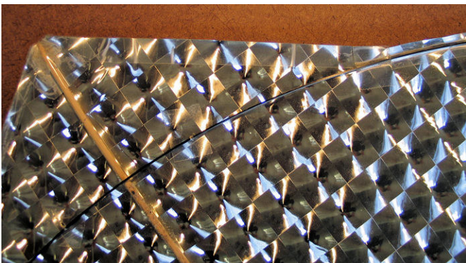
Tape reinforcement along nose leading edge.
